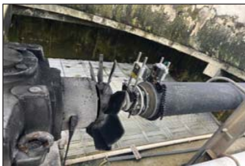
Pict. 2 Check drive shaft alignment gearbox before.
