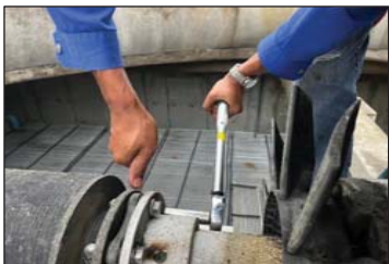
Pict. 10 Tighten torque bolt of drive shaft coupling.
