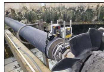
Pict. 7 Adjust drive shaft alignment gearbox after.
