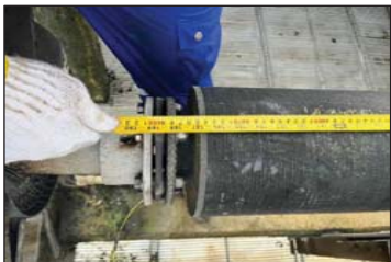
Pict. 9 Check distance between shaft ends after drive shaft.
