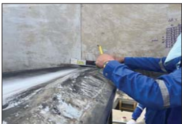
Pict. 11 Measure Tip track, Blade pitch angle, Tip clearance after replace fan blade set.
